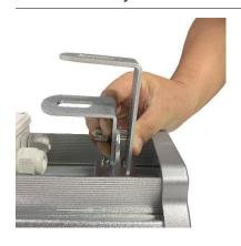
Set of extra long mounting brackets for UBOAT. Suitable for wall/ceiling mounting. The longer mounting brackets allow to mount the luminaire at an angle of 60°.
