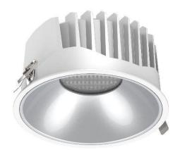
Soft is a high-performance LED downlight with high color rendering CRI90 and low glare UGR<19. Soft is equipped with a deeper mounted LED source with a milky diffuser and an external matte aluminum reflector. Soft is equipped with a Citizen COB LED chip with high efficiency and high color rendering CRI90. The solid aluminum housing has sturdy clamp hinges. Supplied with non-dimmable Tridonic driver and a tool-less connection box for quick connection and throughwiring.
