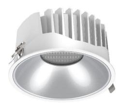
Soft is a high-performance LED downlight with high color rendering CRI90 and low glare UGR<19. Soft is equipped with a deeper mounted LED source with a milky diffuser and an external matte aluminum reflector. Soft is equipped with a Citizen COB LED chip with high efficiency and high color rendering CRI90. The solid aluminum housing has sturdy clamp hinges. Supplied with non-dimmable Tridonic driver and a tool-less connection box for quick connection and throughwiring.
