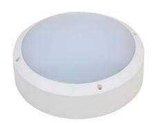
LED luminaire SOLA for wall or ceiling mounting. Impact resistant polycarbonate housing IP65 IK10. Equipped with 'toolless' connection terminals for quick and easy installation. With cable entries along the top and side. With integrated emergency unit 3h 3W 250~300lm.
