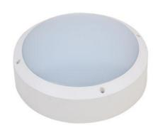
LED luminaire SOLA for wall or ceiling mounting. Impact resistant polycarbonate housing IP65 IK10. Equipped with 'toolless' connection terminals for quick and easy installation. With cable entries along the top and side. With integrated emergency unit 3h 3W, level of light output in case of emergency 10%.
