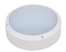
LED luminaire SOLA for wall or ceiling mounting. Impact resistant polycarbonate housing IP65 IK10. Equipped with 'toolless' connection terminals for quick and easy installation. With cable entries along the top and side.
