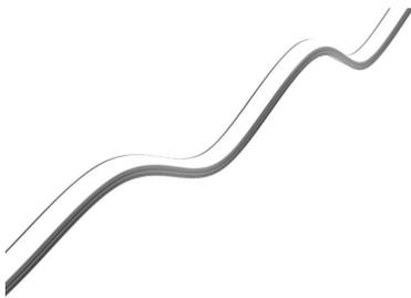
Led profile bendable SLB10 in anodized aluminum AL6063. Complete kit with led profile 2m and milky cover in PC, 2 end caps without cable entry, 2 end caps with cable entry and 4 mounting brackets stainless steel L304 in a handy and sturdy cardboard tube. Maximum bending radius 150 mm.
