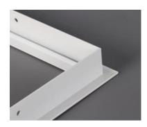
Recessed frame white RAL9016 for hollow ceilings for LED panel 595x595. Outer size 630x630x27mm. Maximum ceiling thickness 25mm.
