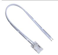
Toolless clamp connector with connection cable 15cm for IP20 monocolor LED strips of 8mm wide. Max. Height 24V 3.5A, cable section 0.5mm $^2$ . Heat resistant up to 105  $^{\circ}$  C.
