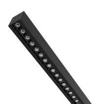
Lineaconnect is a functional aluminum line luminaire in aluminum that can be connected in a simple and fast way. The transparent power cable, invisible brackets for surface mounting and the necessary accessories for in-line coupling are supplied as standard. Type LCU is finished with a black anti-glare screen, which results in an extremely low UGR. Length 1.2m 40W, efficiency up to 90lm/W, standard dimmable 1-10V. A maximum of 20 pieces (40W) can be connected in one line.
