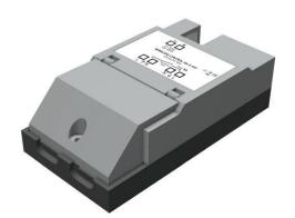
Integraconnect Bluetooth low energy interface IP20 for 0/1-10V drivers. With this interface you can simultaneously control and dim multiple LED luminaires with 0/1-10V driver. Connection voltage 100~240V. Maximum current draw 20mA for 0-10V and 40mA for 1-10V drivers. Integraconnect is 100% compatible with Casambi. Download the free app on the Apple store or Google play. Equipped with internal switching relay 1p 5A. Maximum load 1000W resistive, maximum 500W LED.
