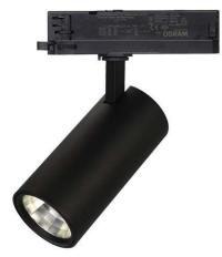
Adjustable track spot for universal Eutrack 3-phase track. Housing black RAL9004 equipped with Citizen LED chip with high color rendering CRI90 and Alanod reflector 30° with an efficiency of 97%. Powergear rail adapter with integrated flickr free Osram driver, not dimmable. Lifespan 50;000h L80B20, warranty 5 years.
