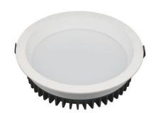
LED downlight Compact with compact installation height. Equipped with Osram SMD3030 LED chips with color rendering CRI90 in a solid aluminum housing with clamping springs and white opal diffuser with even light distribution. Supplied with universal Unidriver dimmable with TRIAC, 1-10V, DALI2 or push. Unidriver has an inrush current of only 2A and does not use a PWM output signal during dimming, but amplitude dimming = no flicker or stroboscopic
