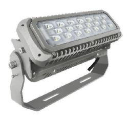
Industrial floodlight Brightmaster 2 with 110° lens. Gray aluminum IP65 housing for even better cooling. Interpon coating for corrosive environments. Directional LED modules with Lumileds 3030/5050 and a Meanwell HLG driver. Equipped with junction box and 1.3m cable H05RN-F.
