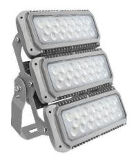
Industrial floodlight Brightmaster 2 with 25° lens. Gray aluminum IP65 housing for even better cooling. Interpon coating for corrosive environments. Directional LED modules with Lumileds 3030/5050 and a Meanwell HLG driver. Equipped with junction box and 1.3m cable H05RN-F.
