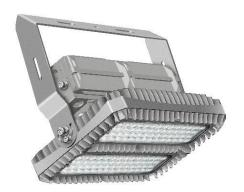
Industrial floodlight Brightmaster 2 with 90° lens. Gray aluminum IP65 housing for even better cooling. Interpon coating for corrosive environments. Directional LED modules with Lumileds 3030/5050 and a Meanwell HLG driver. Equipped with junction box and 1.3m cable H05RN-F.
