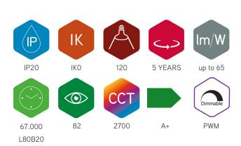
LED flex 120MLED is equipped with 120 LEDs type SMD2835 per meter and suitable for universal use in all kinds of applications. Thanks to the very short sections of 16.66 mm, customization becomes easier and any desired length can be achieved. Connection voltage 24VDC, to be shortened every 16.66 mm. Color rendering CRI82, light beam 120°. Lifespan 50.000h L80B20. Equipped with pre-soldered connection cables of 30 cm on both sides.
