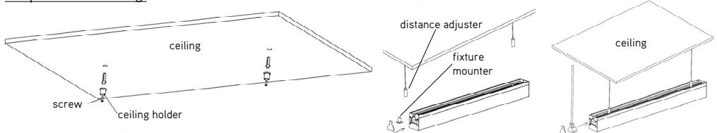
Mount the ceiling holders of the pendulum set at a distance of your choice. The pendulum set can be attached over the entire length of the fixture. Slide the steel cable through the screw of the ceiling holder and attach it.
