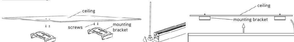
Put the mounting brackets at a distance of your choice. The brackets can be mounted over the entire length of the fixture.
