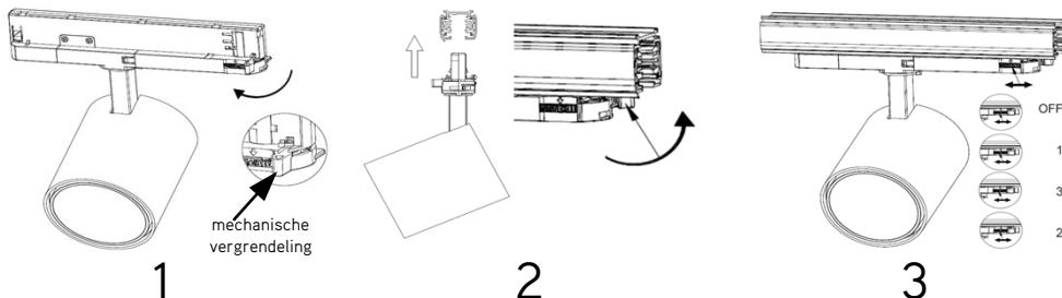
Make sure the mechanical lock is open as shown above.
